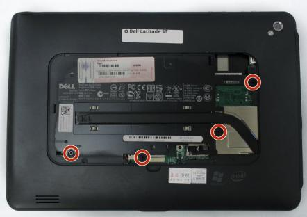
Using a Phillips #0 screwdriver, remove the four 6mm screws attaching the inside panel to the device.
