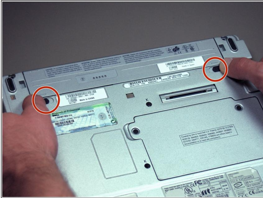
**⚠** Before removing the battery from the laptop, make sure the power is off.
