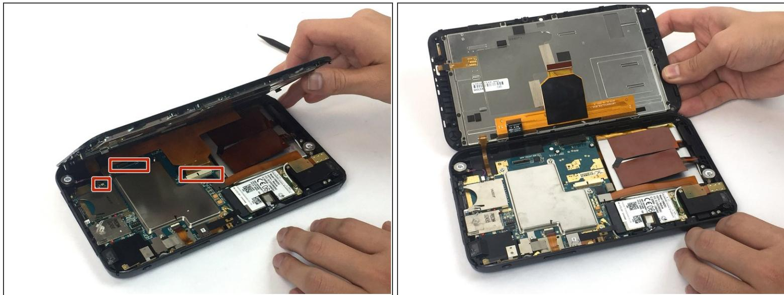
**i** Ribbon cables are very sensitive and prone to breaking
