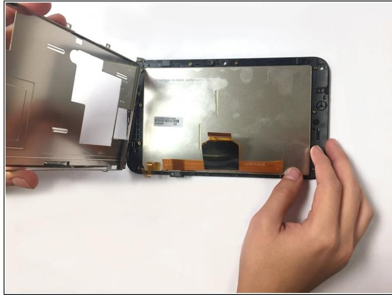
! Ribbon cables are very sensitive and prone to breaking
