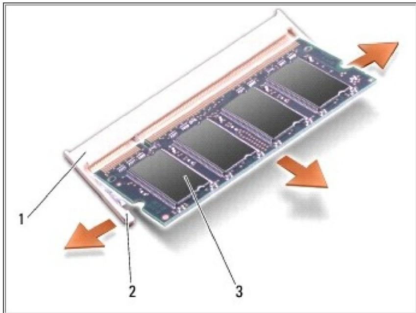
**NOTICE:** To prevent damage to the memory module connector, do not use tools to spread the memory module securing clips.
