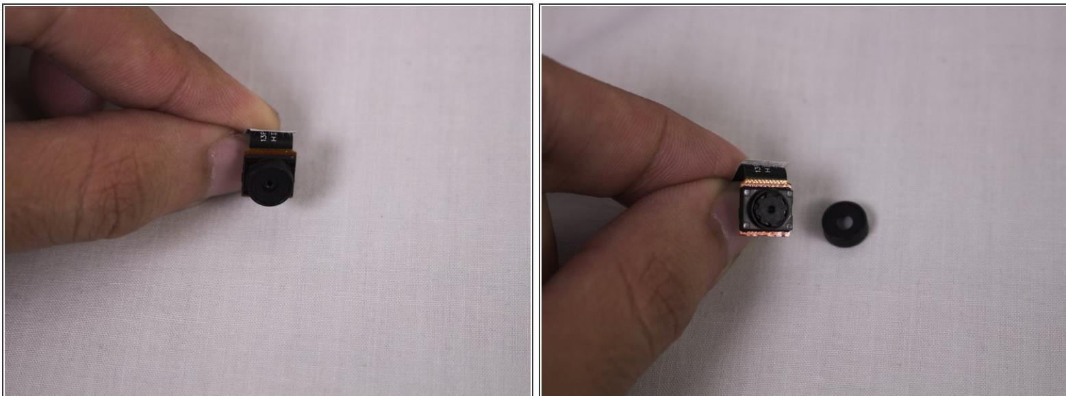
*(i)* Take caution when removing the front camera with the rubber cover. The cover can easily fall off from any slight movement.
