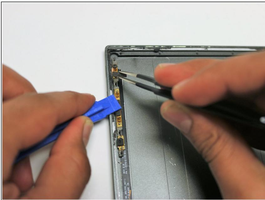
*(i)* Just like the volume button, you want to make sure that you hold the left side of the tablet open with a plastic opening tool so that you will be able to take out the power button.
