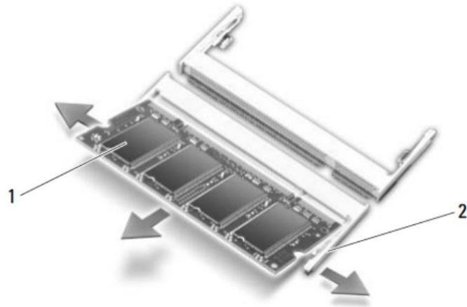
**NOTICE:** To prevent damage to the memory module connector, do not use tools to spread the memory-module securing clips.
