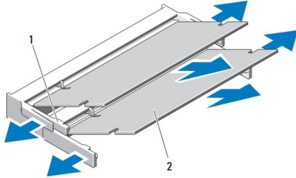
**NOTICE:** To prevent damage to the memory module connector, do not use tools to spread the memory module securing clips.
