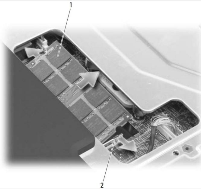
*(i)* **NOTICE:** To prevent damage to the memory module connector, do not use tools to spread the memory-module securing clips.
