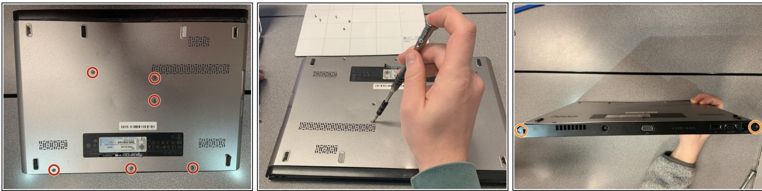
! Back up the memory to an external drive and power off the laptop before starting.
