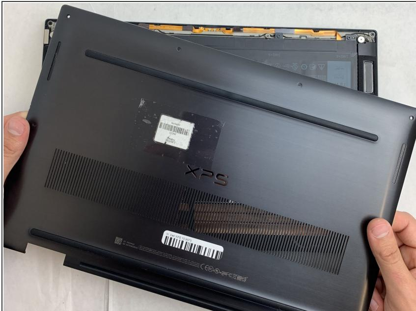
⚠ Make sure all screws are removed before you lift the panel to prevent any damage from occurring.
