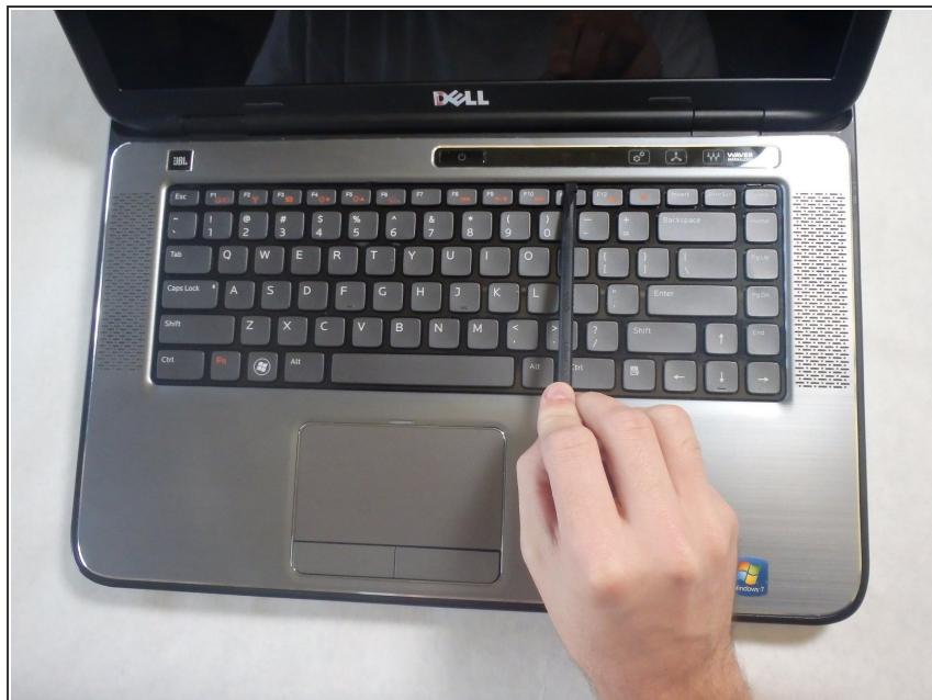
**i** Prior to prying up on the cover, you may have to first remove one screw located inside the battery compartment (M2X3) and release the two (2) latches or you'll snap the cover.
