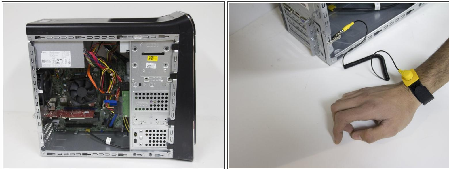
**⚠** Before working on the internal components put on the Anti-Static wristband to avoid an electrical shortage.
