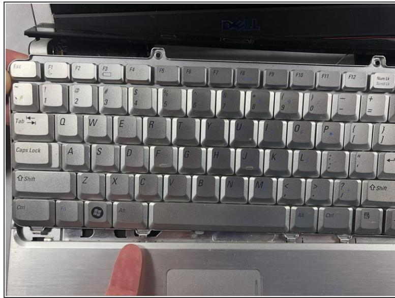
⚠ When removing this piece lift slowly as there is a cord underneath that connects to the keyboard.
