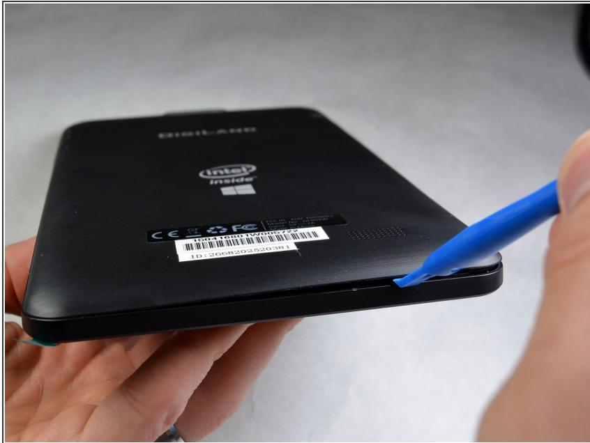
**⚠** Please be aware that removing the back panel from the tablet could cause damage to the back or front panel.
