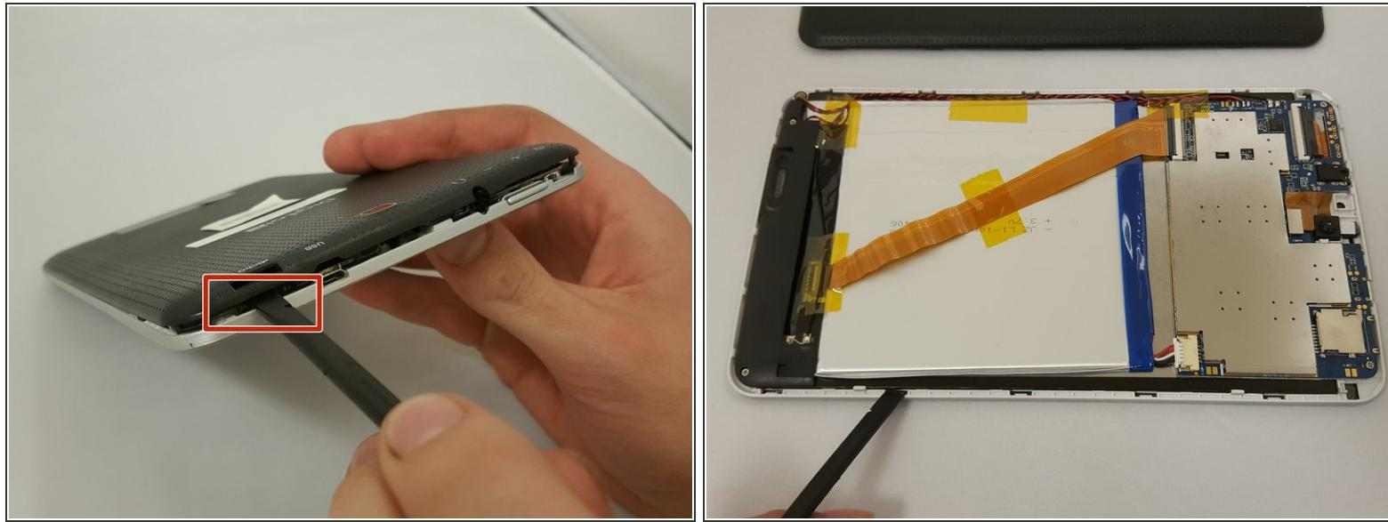
**⚠** Do not use a lot of force as it can break the clips or the back panel.
