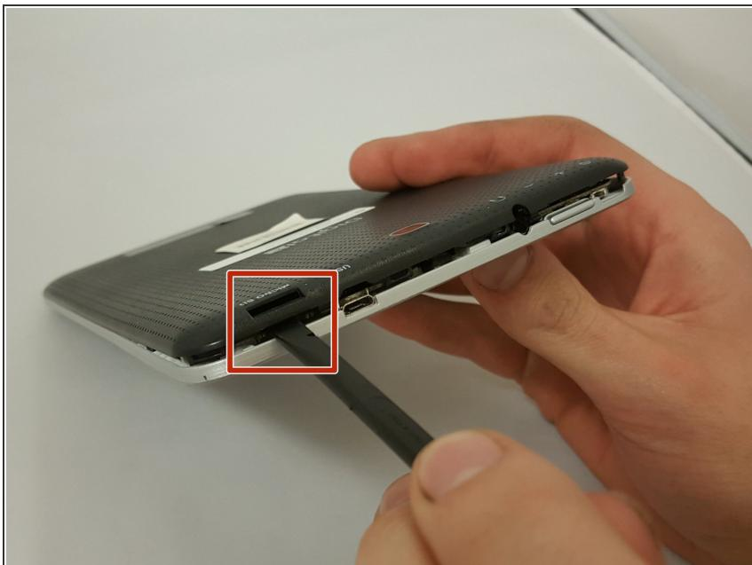
**⚠** Do not use a lot of force as it can break the clips or the back panel.
