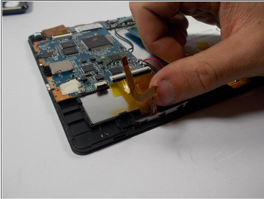
⚠ Make sure to separate the volume button's cable from the cable connecting the motherboard to the screen
