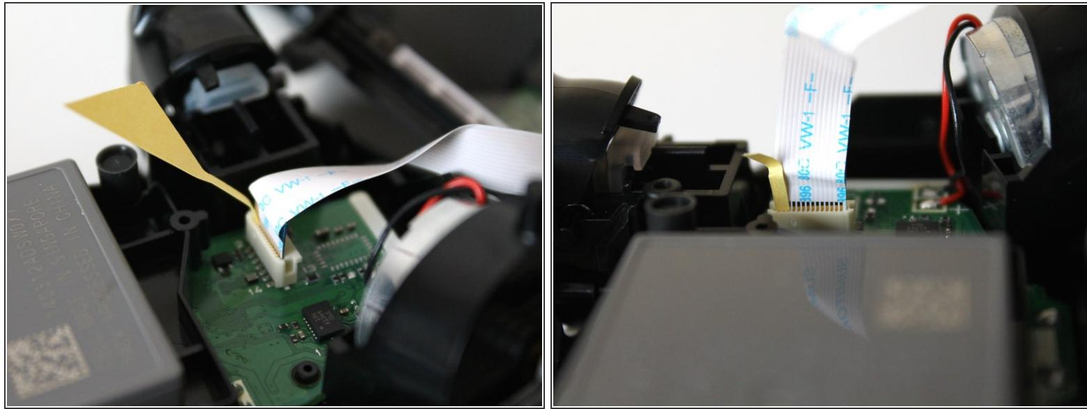
⚠ Don't twist the ribbon cable when inserting it.
