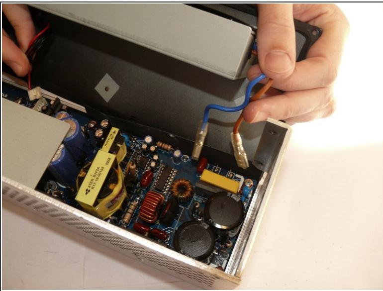
**⚠ Caution:** The circuit board contains many capacitors that could cause serious injury if touched. If possible, use a [capacitor discharge probe](#) to safely rid the capacitors of dangerous charges.
