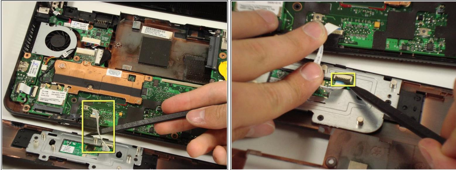
! Careful lifting up the cover because the track pad is still attached.
