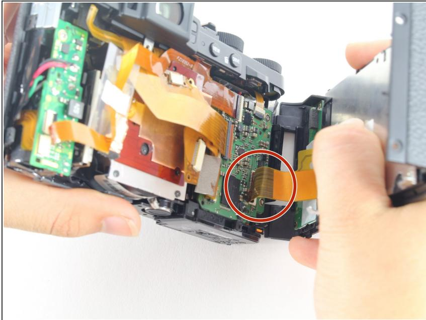
**⚠** Do not pull hard when removing the backing because it could rip the orange strip attached to the motherboard.
