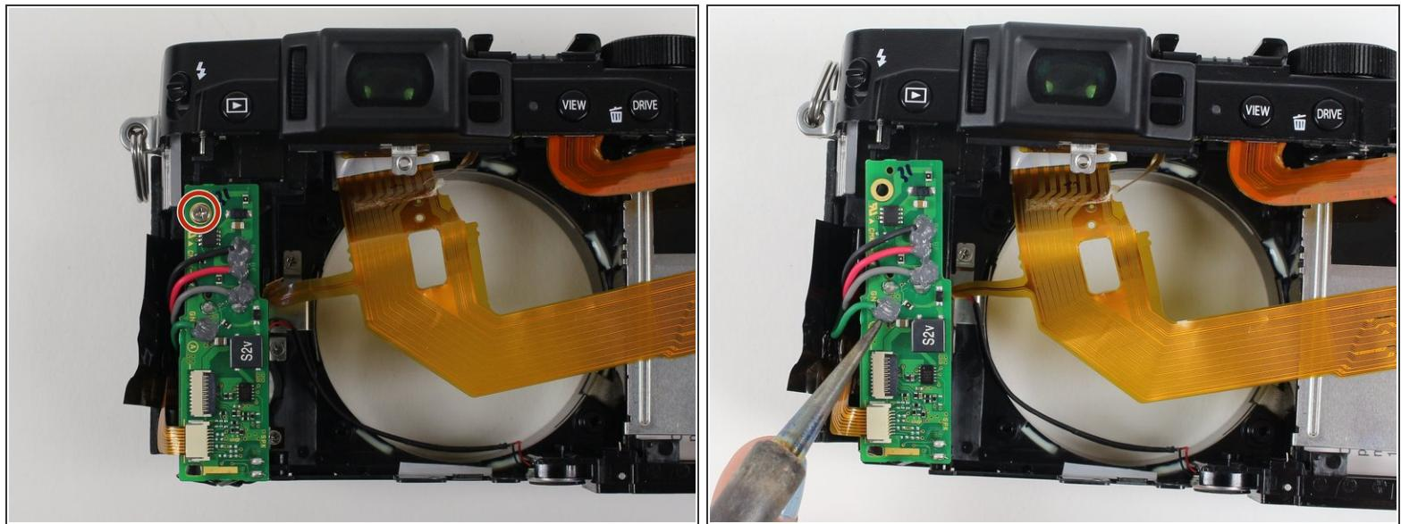
⚠ Do not touch the leads on the capacitor below the green circuitboard because they can shock you.
