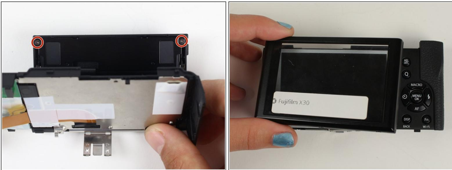
*(i)* To remove the LCD screen, look at the back of the tiltable screen plate.
