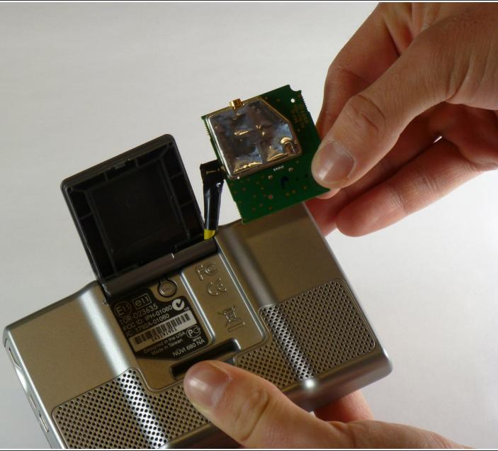
**⚠** The yellow wire is connected to the motherboard, so you cannot disconnect it until you finish opening the device.
