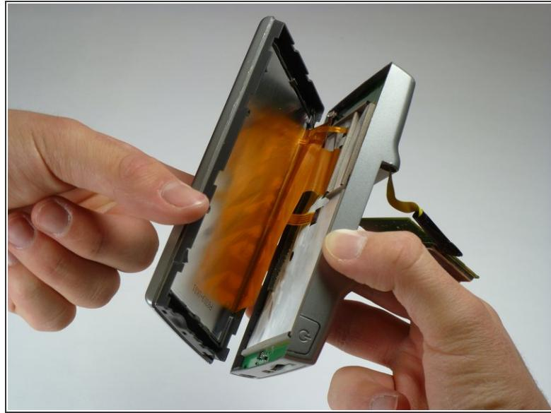
! Gently pull apart the front and back of the device. The front and back are still connected by ribbon cables.
