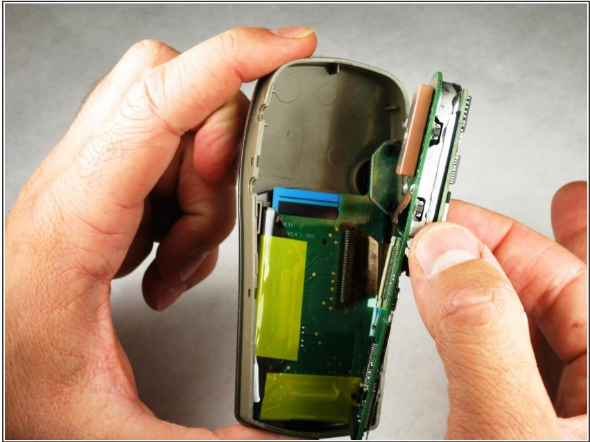
☞ There are no screws holding the motherboard in place.
