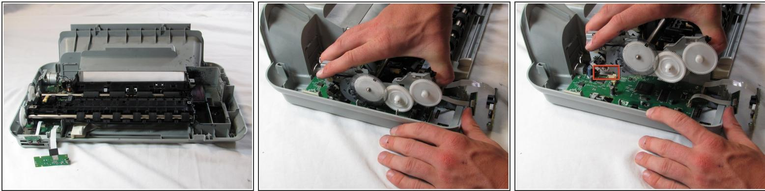
ⓘ This step can be performed with out rotating the printer, but we have rotated the printer for clarity.
