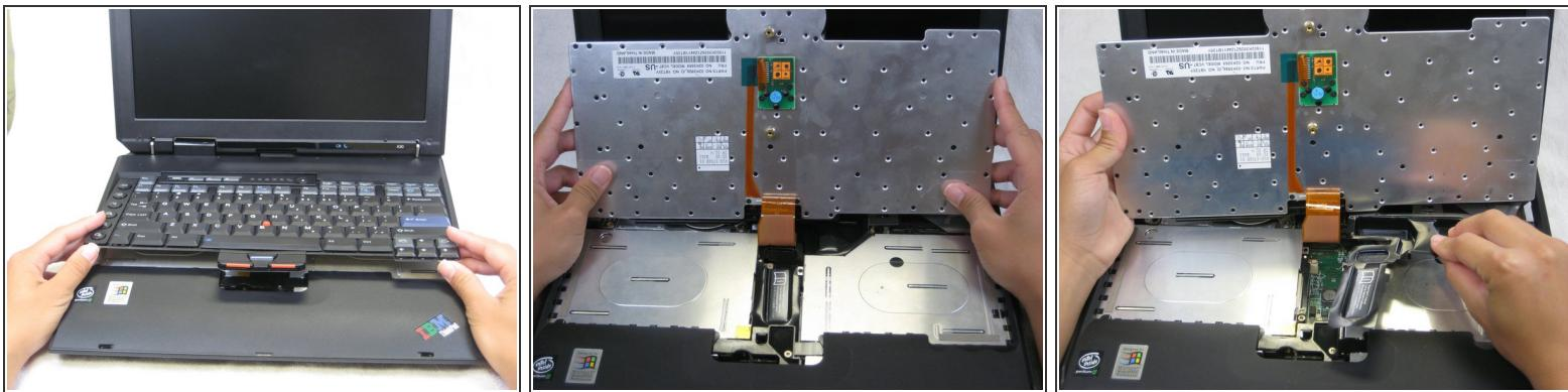
**⚠** Be careful not to pull out the keyboard carelessly; there is a connector underneath it!
