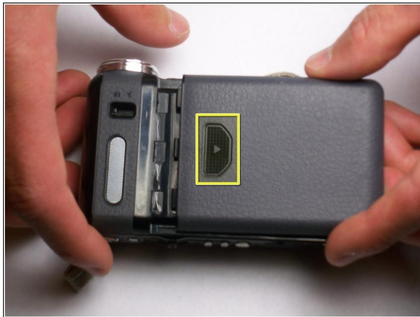
On the back of the camcorder, the side opposite of the flip-out screen, there is a section of grooved plastic with a small arrow.
