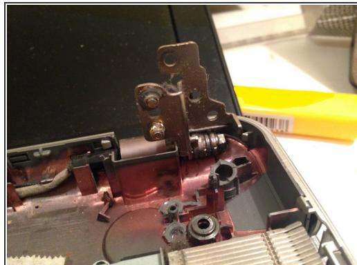
① Repairing the broken hinge [detailed photo]
