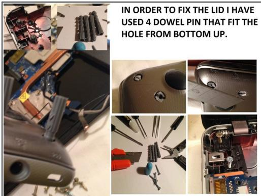
IN ORDER TO FIX THE LID I HAVE USED 4 DOWEL PIN THAT FIT THE HOLE FROM BOTTOM UP.
