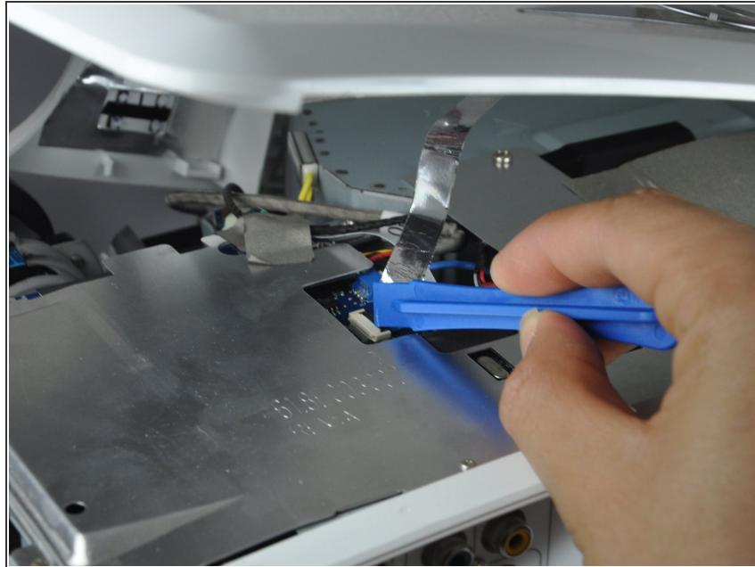
**⚠** When removing the cover, be cautious of the ribbon connecting the top buttons to the main circuit board. The ribbon must be disconnected before proceeding.
