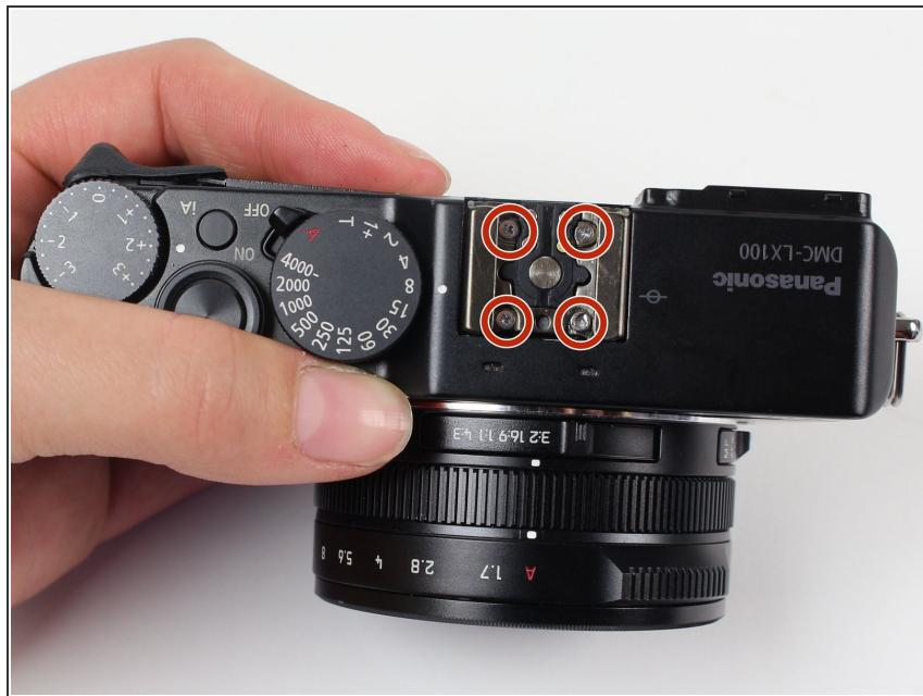
⚠ Some of these screws may have adhesive to keep the camera from being taken apart so push hard with the screwdriver and turn slowly to avoid stripping screws.
