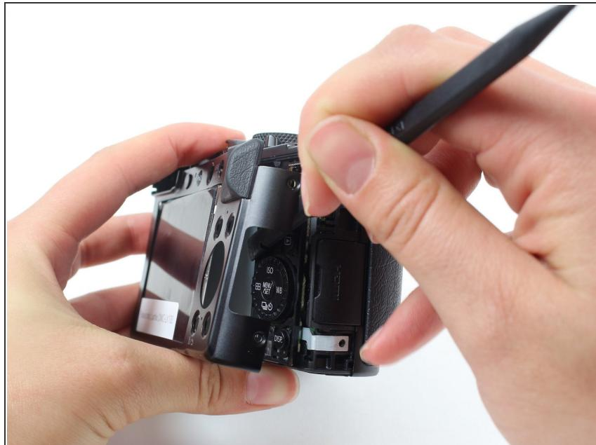
⚠ There may be adhesive holding the back on, so pry carefully to not break any of the ribbon cables underneath.
