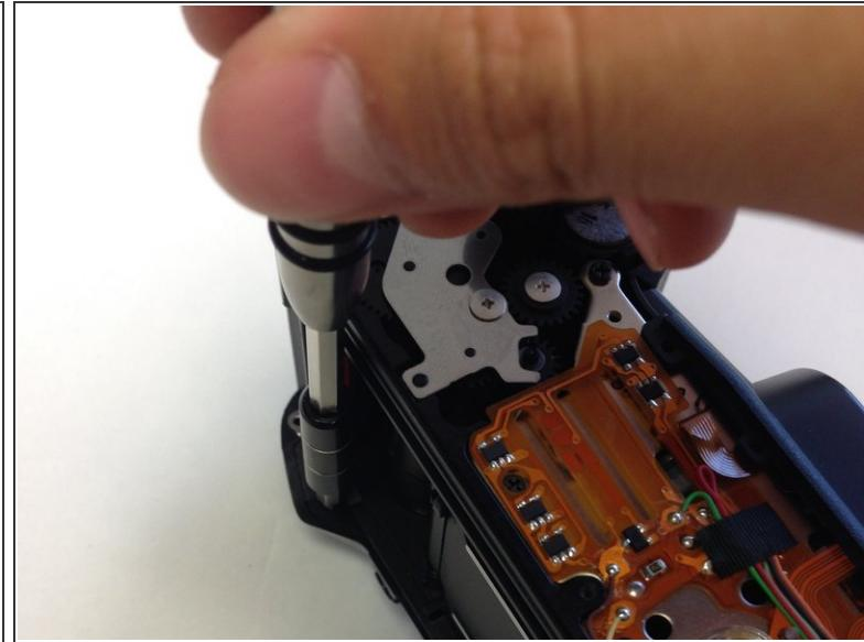
ⓘ With the camera lens face down, locate the screw under the overhanging piece of the top casing on the right side of the back panel.
