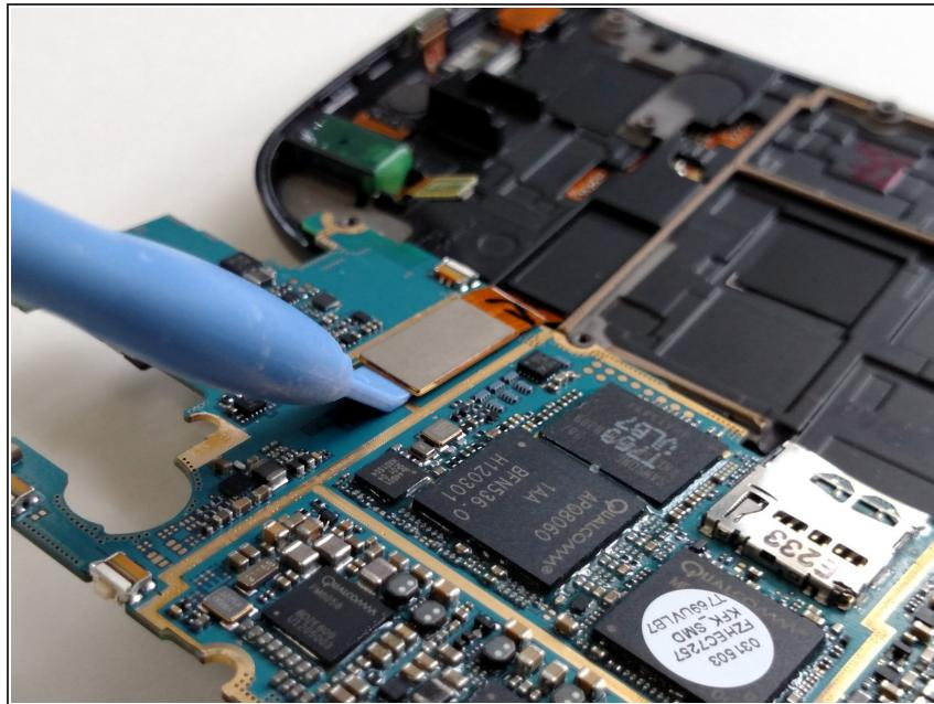
*(i)* Flip the motherboard over to access the last ribbon cable connector.
