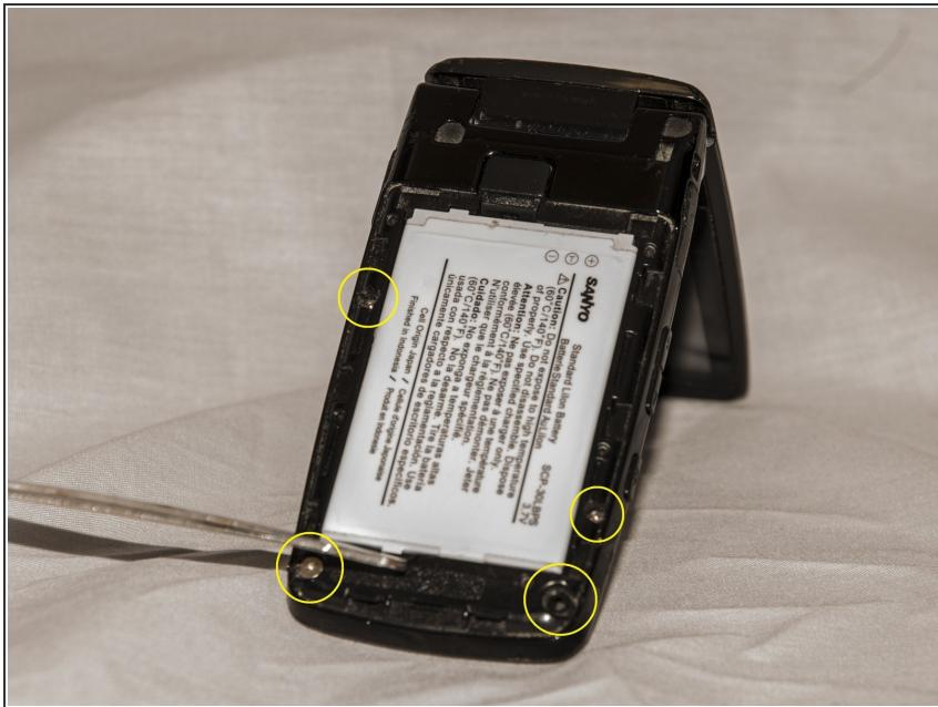
**⚠** This task can be difficult. This phone has several specialized screws that are engineered to prevent removal.
