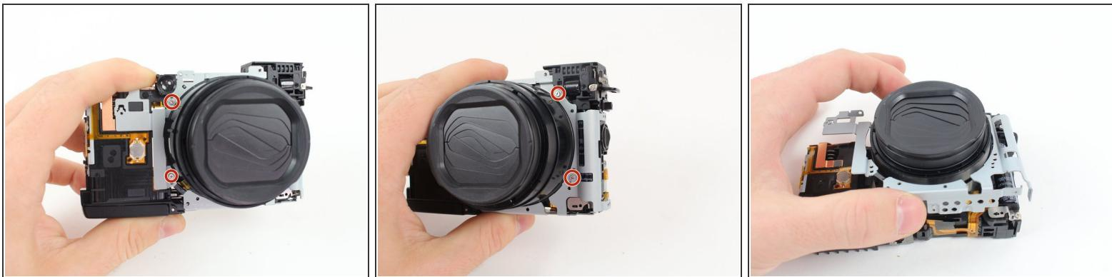
! Lay the camera on a flat surface while performing these steps because removing the frame causes the camera to fall apart.
