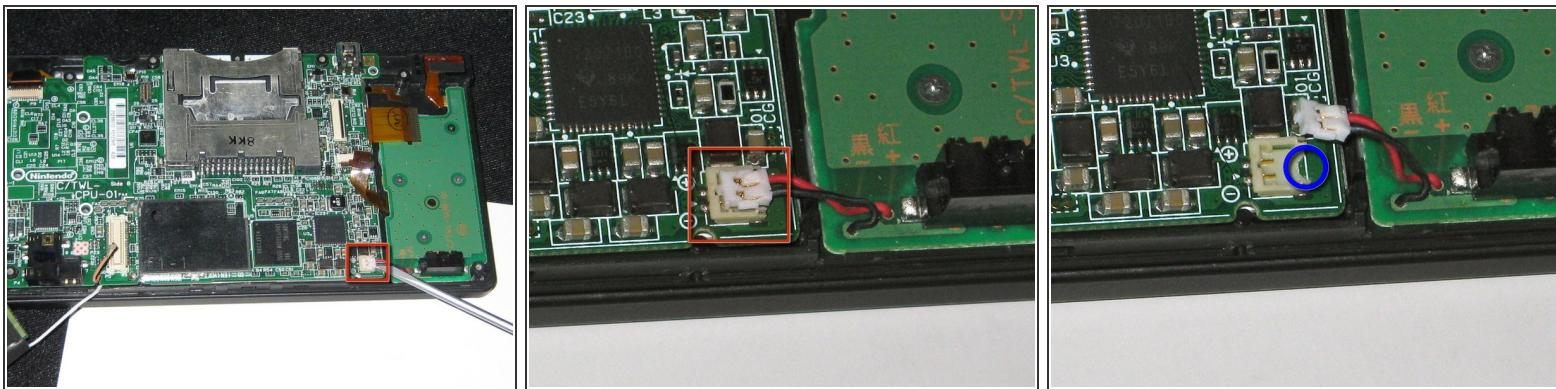
**⚠** The power connector (with red and black wires) is difficult to remove without damaging it, unless you take a moment and understand how it works. Look at all of the photos for this step before continuing.
