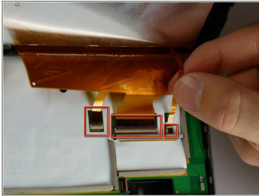
**⚠** Do not remove the ribbon cables without lifting the latch or the cable will be damaged.
