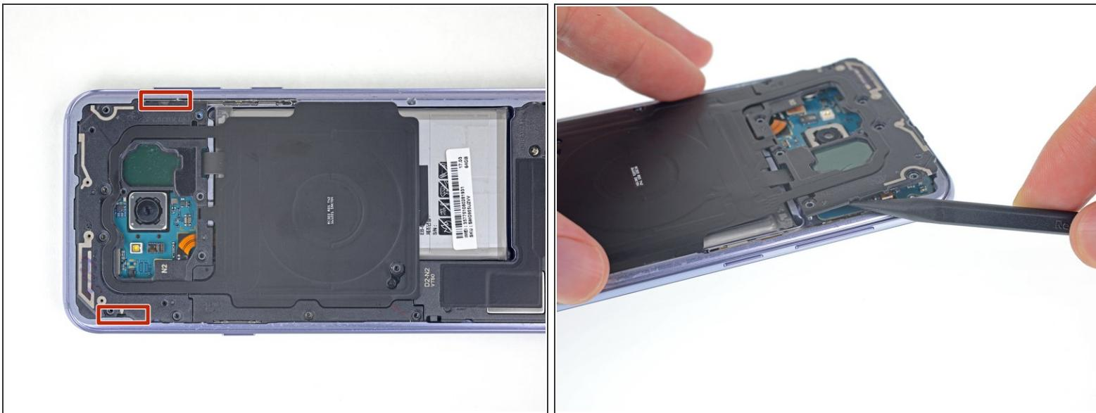
*(i)* The wireless charging coil + antenna assembly is also secured with small plastic clips.
