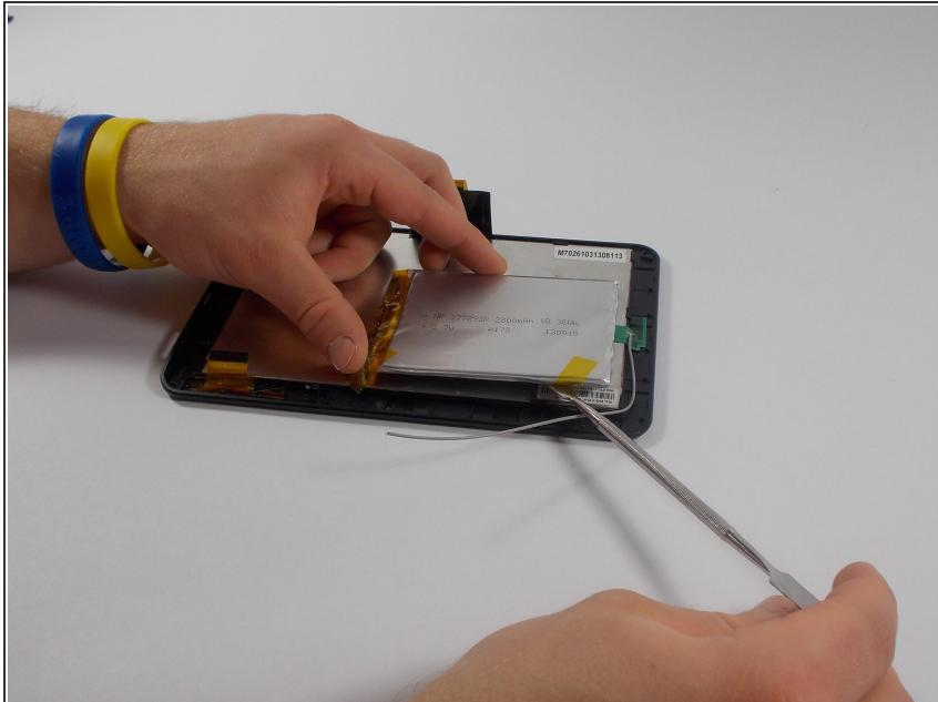
● Using a metal spudger, carefully pry the battery away from the digitizer.
