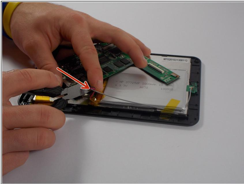
⚠️ Using wire cutters, cut only the **gray** wire.
