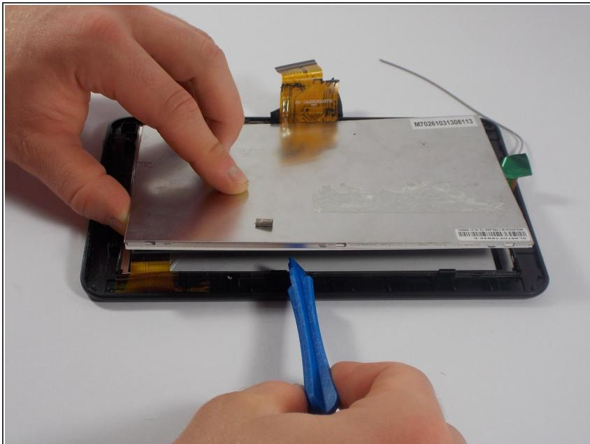
*(i)* The best way to remove the digitizer is to use a plastic tool and pull back the clips so that it can lift out.
