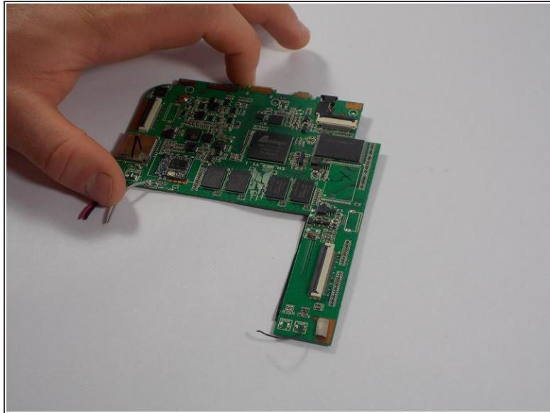
⚠ Using wire cutters, cut the red, black, and grays wires. Leave enough wire to be re-soldered back if possible.
