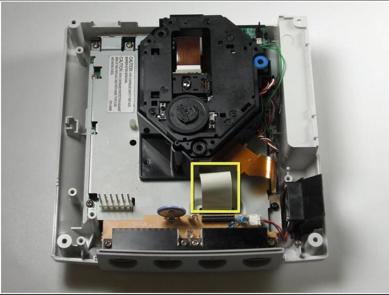
! Be gentle with the white controller cable as it can be a bit fragile.
