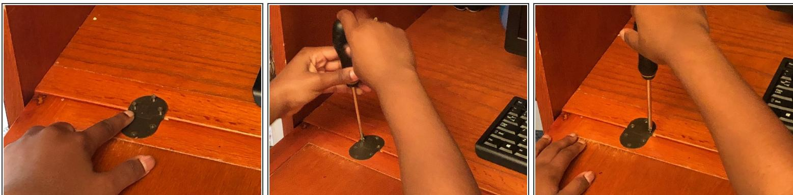
⚠ Have one person hold the drop-front panel in place and another person screw the hinges in place.
