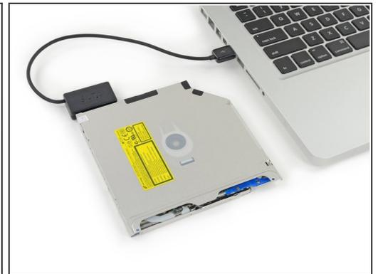
**i** Don't ditch that drive! You can still use your optical drive externally with the help of our [SATA Optical Drive USB Cable](#).
