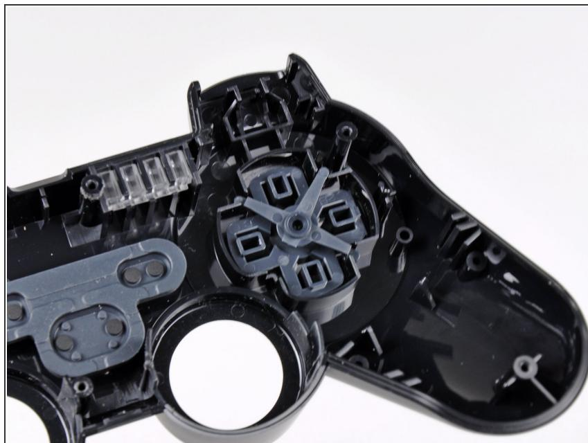
*i* The D-pad has a three-armed plastic piece that must be installed as shown before installing the rubber button pad for it to work properly.
