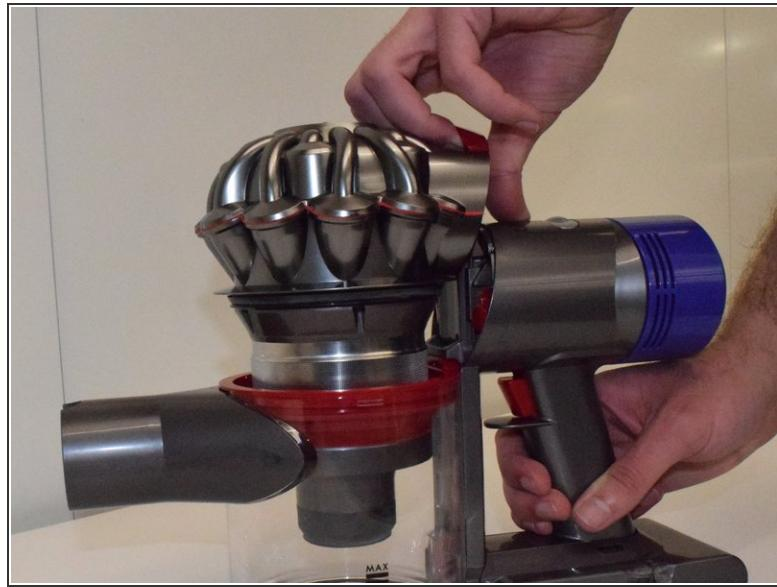
*(i)* First, make sure the device is unplugged and detach the wand from the main unit.
