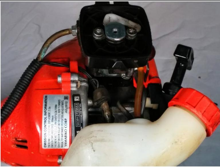
**⚠** Make sure to empty any gas in the tank into an appropriate container before beginning to work on equipment.
