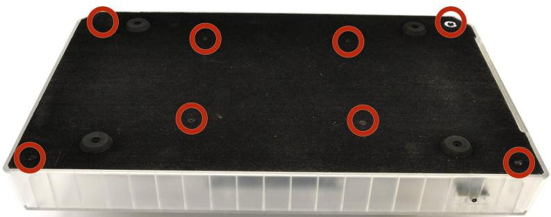
**⚠** Because of the protruding joystick on the top of the controller, make sure to work on a soft surface, or prop the controller up to avoid stress on the joystick.
