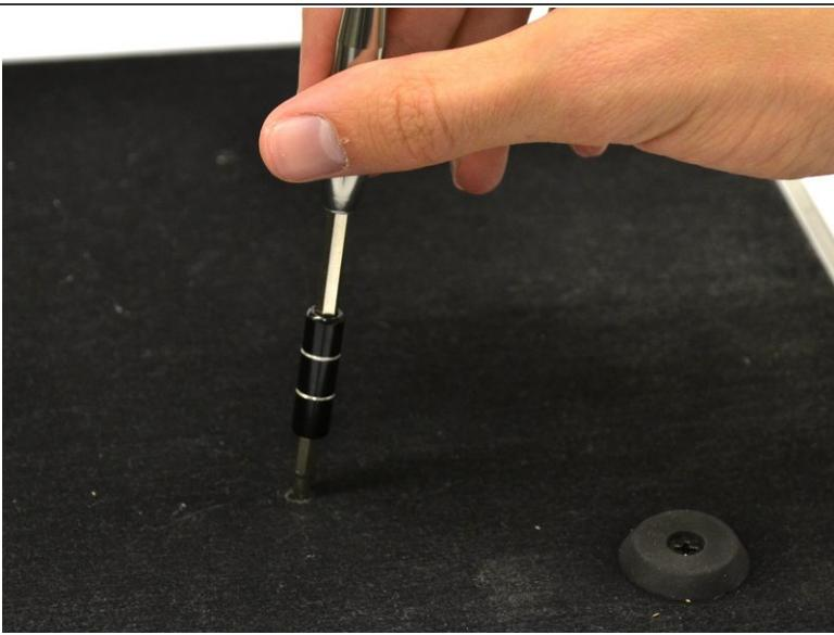
**⚠** Because of the protruding joystick on the top of the controller, make sure to work on a soft surface or prop the controller up to avoid stress on the joystick.
