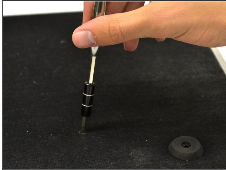
**⚠** Because of the protruding joystick on the top of the controller, make sure to work on a soft surface or prop the controller up to avoid stress on the joystick.
