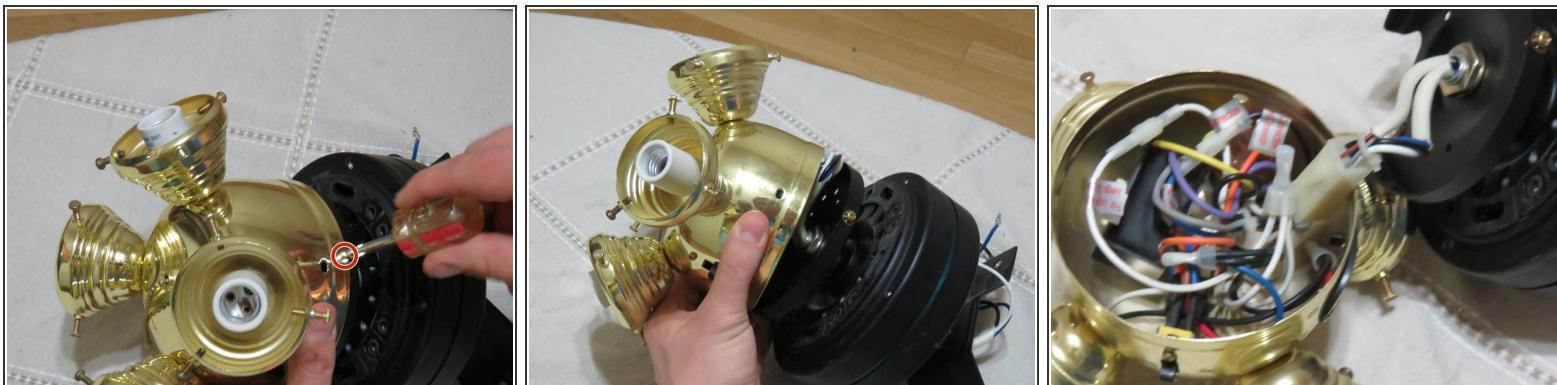
**⚠** Remove light bulbs before working on switch housing.
